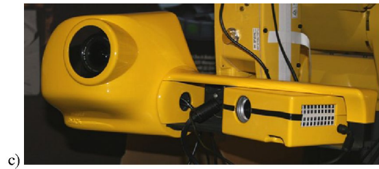
Figure 2: Two exemplary measurement heads developed for CH objects 3D documentation: a) CAD model and b) a photo of SAPO measurement head, c) OGX|AUTOMATED measurement head
