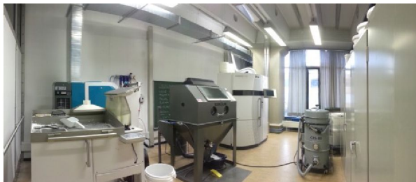
Figure 2: SLS (selective laser sintering) machine with peripheral equipment
